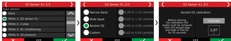
The free-air calibration also can be performed through FTManager Software. To reach the calibration screen, with an open map, go to Sensors and Calibration in the left menu, then enter Inputs and select the channels where the Alcohol O2 analog outputs are connected.
